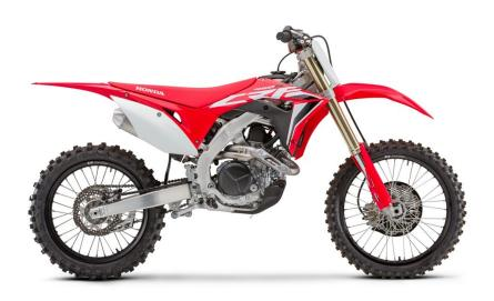
Honda's mighty CRF450R is now equipped with Honda Selectable Torque Control, hand-in-hand with optimisation of the PGM-FI and HRC Launch Control mapping. The suspension features revised settings, and there are also updates to the rear brake and graphics.
