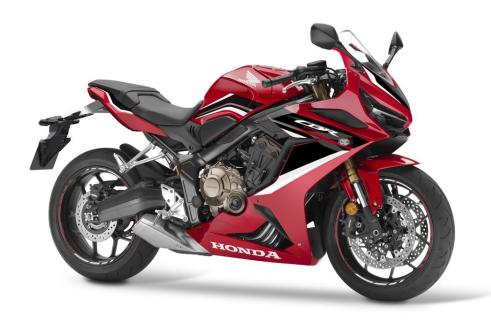
Model updates: Honda's versatile middleweight sports bike gains Showa's 41mm Separate Function Big Piston forks, plus EURO5 compliance for the high-revving four cylinder engine. Other updates include improved LCD dash, revised headlight reflectors, USB Type-C socket under the seat and updated graphic treatment.
