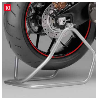
10 Paddock Stand A tilting tubular steel stand that lifts and holds the motorcycle by the end of its swingarm to facilitate cleaning and rear wheel maintenance.
