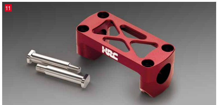
11 Oversized Handlebar Holder The same design as those used on the HRC factory bikes, this Handlebar Holder allows oversized 28mm (1 1/8 inch) handlebars to fit the standard triple clamp. Featuring the HRC logo and finished in red aluminite for increased durability, the set includes chromium molybdenum steel bolts for increased rigidity. Not available for the CRF150R.
