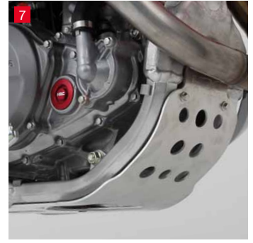
7 Aluminium Bottom Skid Plate An aluminium skid plate featuring the HRC logo that bolts to the underside of the frame to protect the engine crankcase from stones, and helps to slide off cased jumps. For the CRF450R & CRF250R only.
